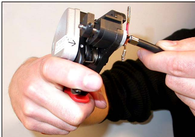
figure 3.14: Cutting a fiber (3)
