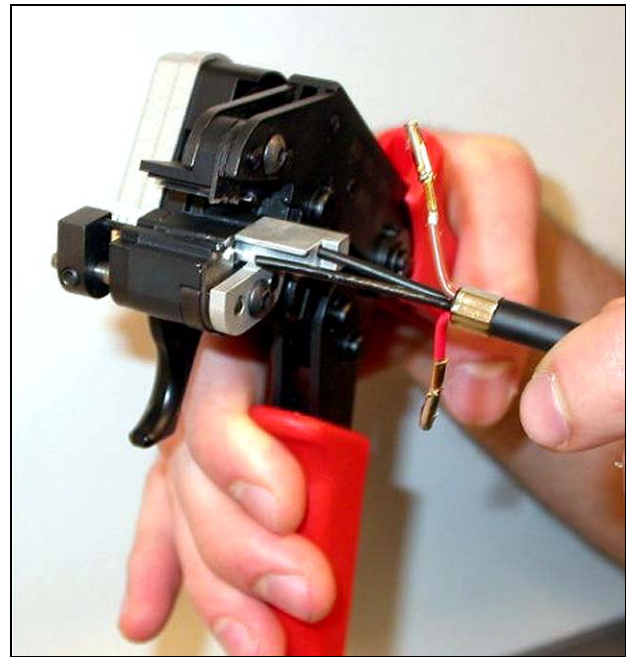
figure 3.12: Cutting a fiber (1)
