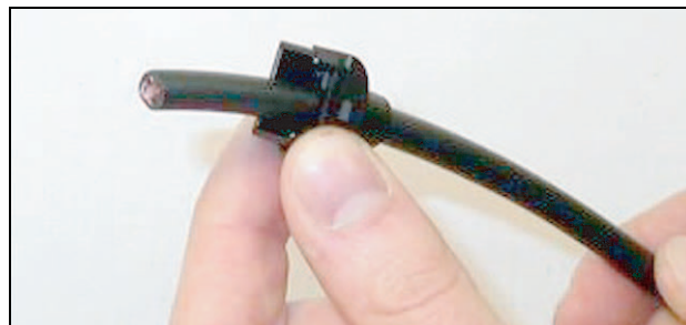
figure 3.2: Back housing on cable
