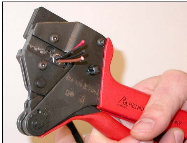
figure 3.5: Crimping the bush
