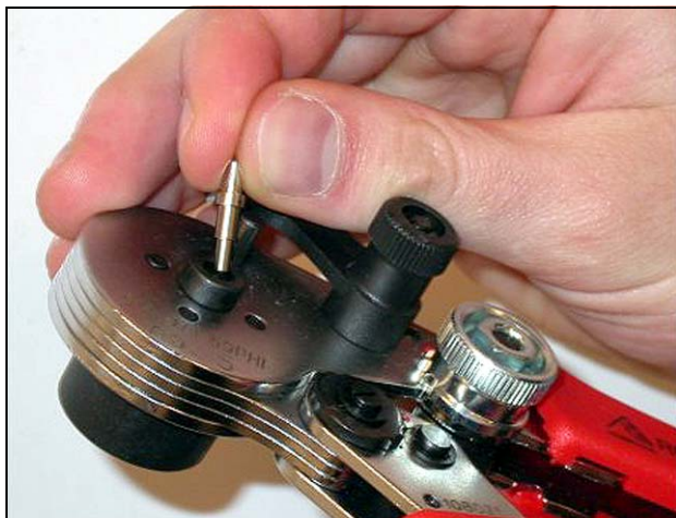
figure 3.17: Inserting a ferrule
