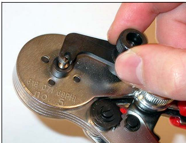
figure 3.18: Locking a ferrule
