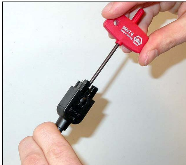
figure 3.33: Tightening the Torx screw
