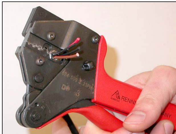
figure 22.9: Crimping the bush
