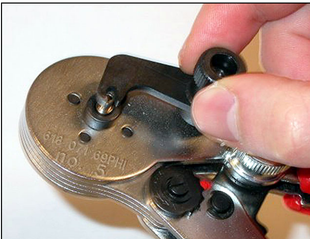
figure 22.22: Locking a ferrule
