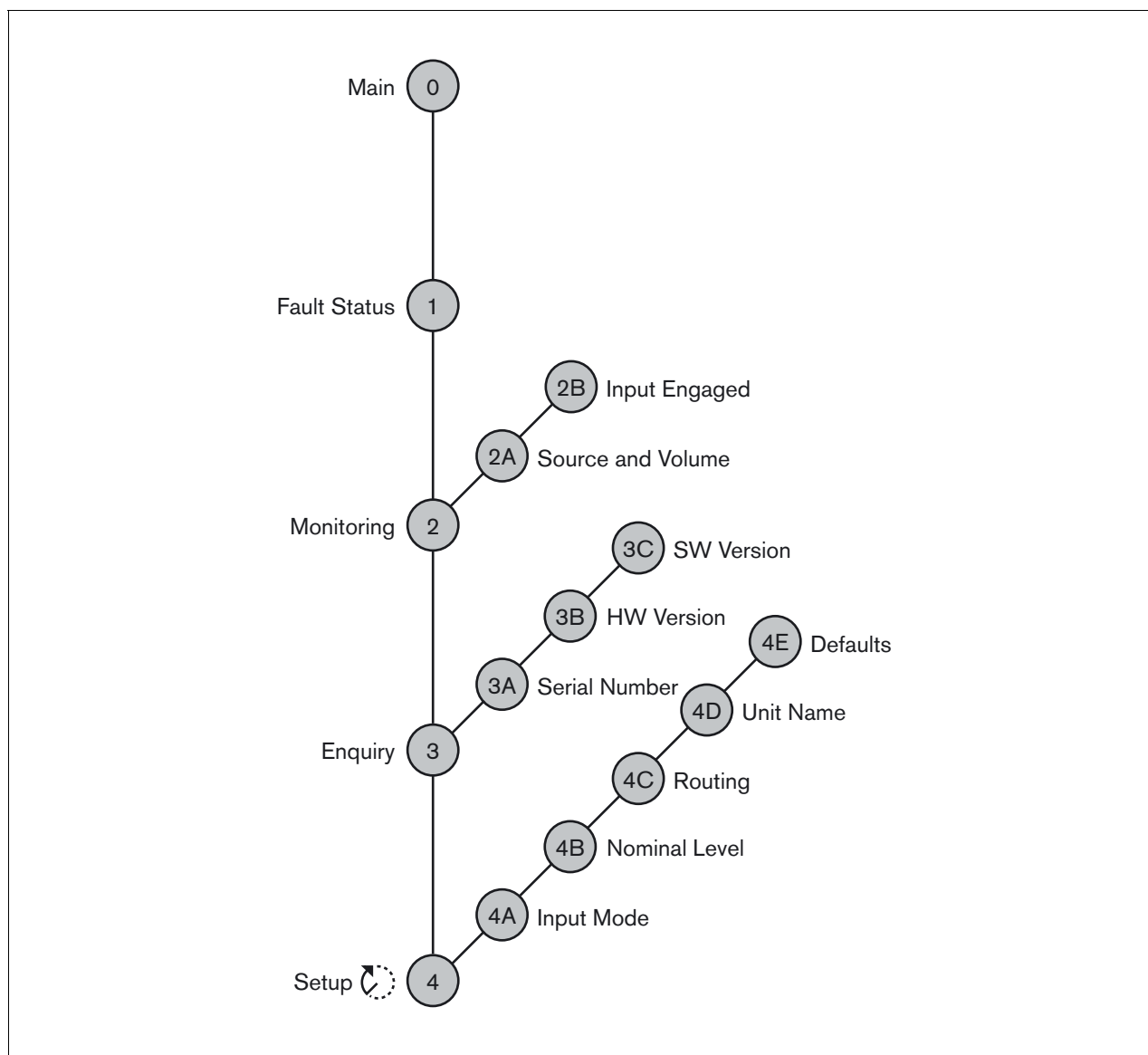
figure 10.8: Structure of the analogue audio expander front panel menu
