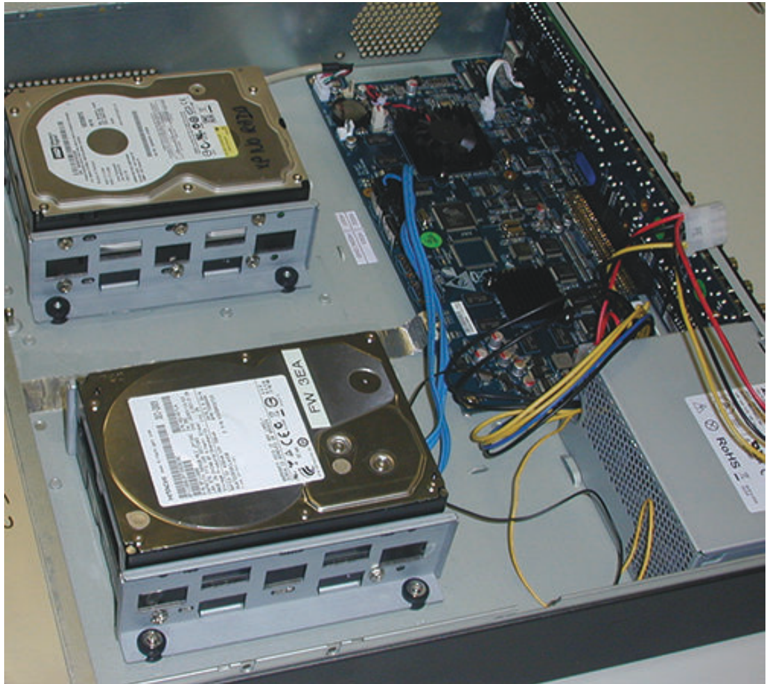
Figure 11.10: Install HDD 3 and 4
