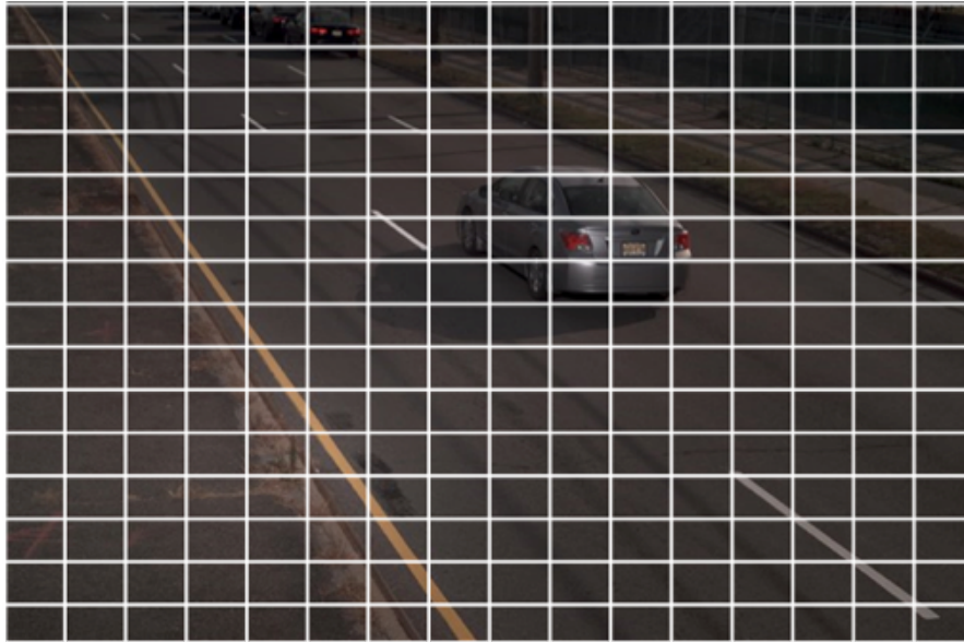
Figure 2: I-Frame divided into blocks using H.264
