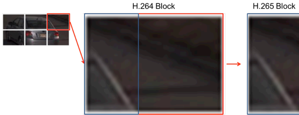
Figure 10: H.264 coding block with reduced size H.265 block
