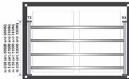
Figure 1: Example of a barrier 5100B or 5100N installed on a door or a window with optional profile extension
