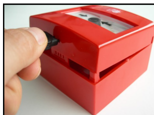
Picture 10 - removing the front device from the back box - surface mounting, but the same principle applies to flush mounting
