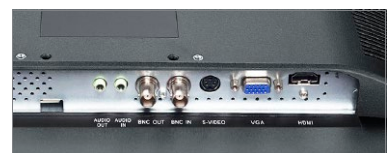
Video versatility, including VGA, HDMI, S-Video and BNC In/Out
