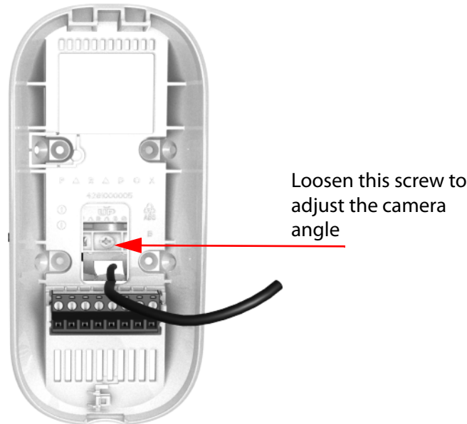
Figure 14 – Screw Location to Adjust Camera Angle
