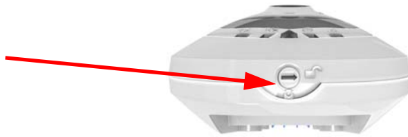
Figure 62 – Separating the Module from the Camera Housing
