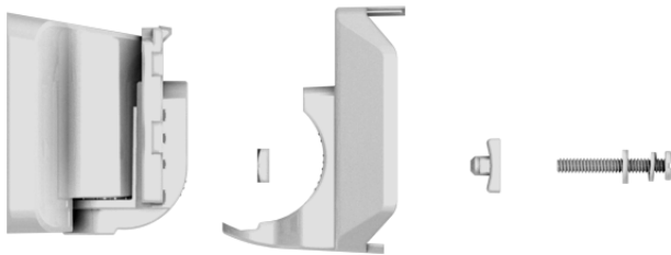
Figure 61 – Screw the Slider, HD77 Camera Housing and Back Housing Together
