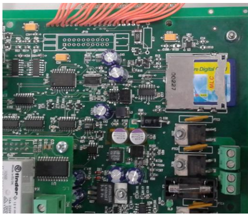
Fig. 4.4.1 f) SD card location on the main board
