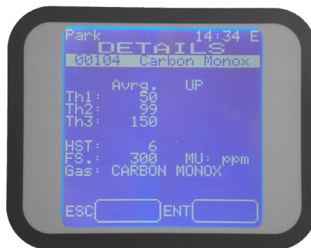
Figure 42) Detector details screen in “Engineer” level
