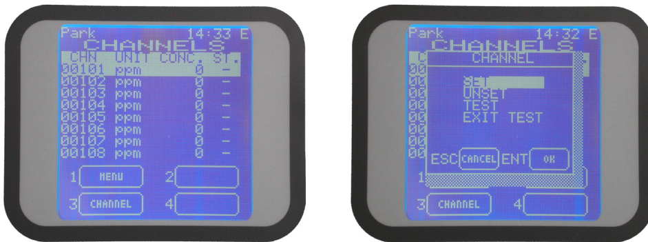
Figure 40) Detectors screen and options available pressing 3-Channel
