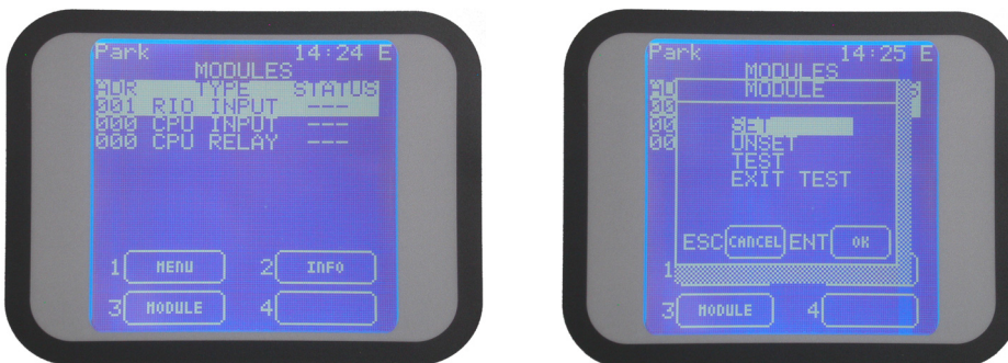
Figure 36) Modules screen and available options pressing 3-Module
