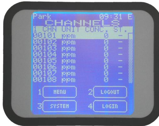
Figure 19) Typical NORMAL state screen.
