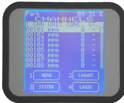
Figure 20) Typical NORMAL state screen.
