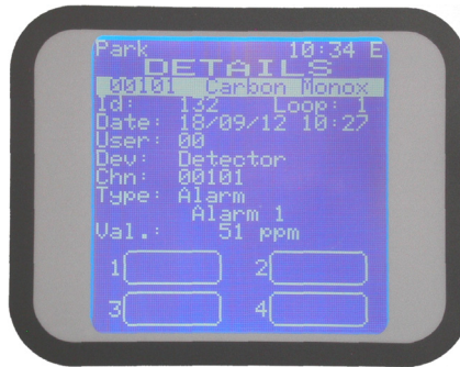
Figure 22) ALARM details screen.
