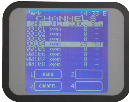
Figure 41) Screen with channel in “Test”
