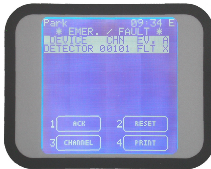
Figure 28) Active events screen with fault only
