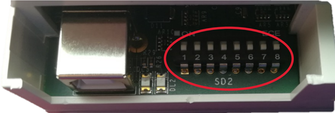
Figure 7) Dip switch series for baud rate settings
