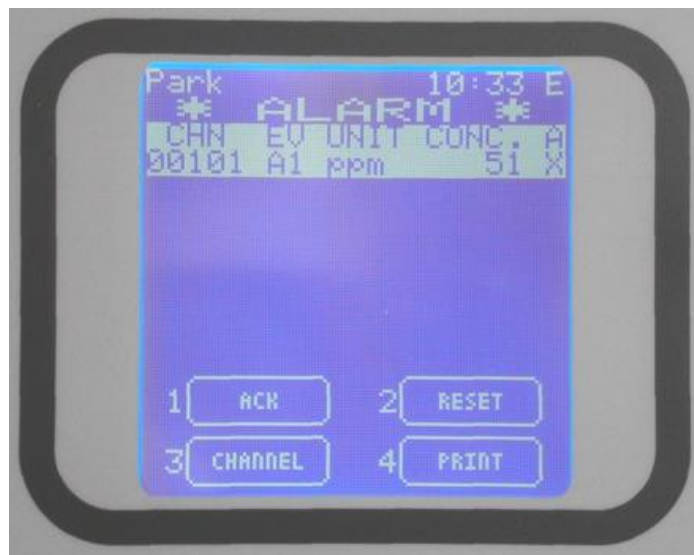
Fig. 3.2.1.b) Typical ALARM state of the ACTIVE EVENTS screen.
