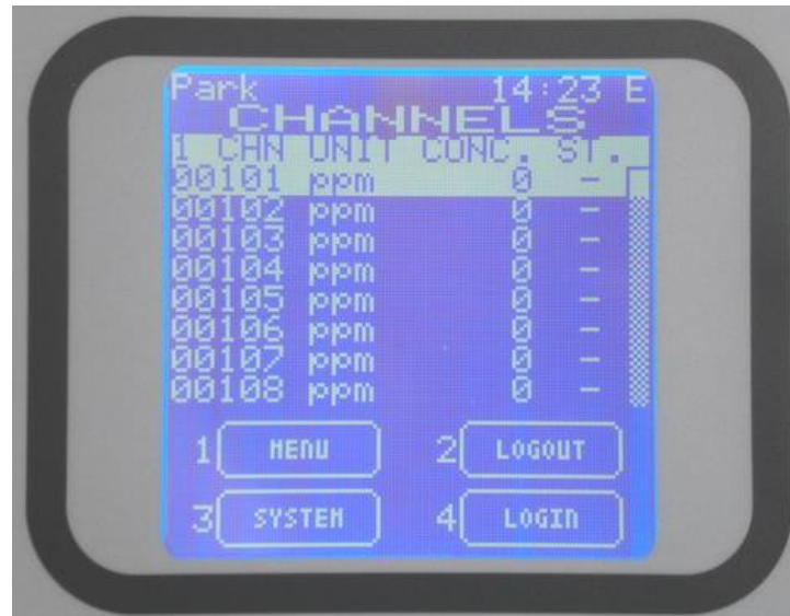
Fig. 3.7 b) NORMAL state screen with the “E” in the right and upper corner
