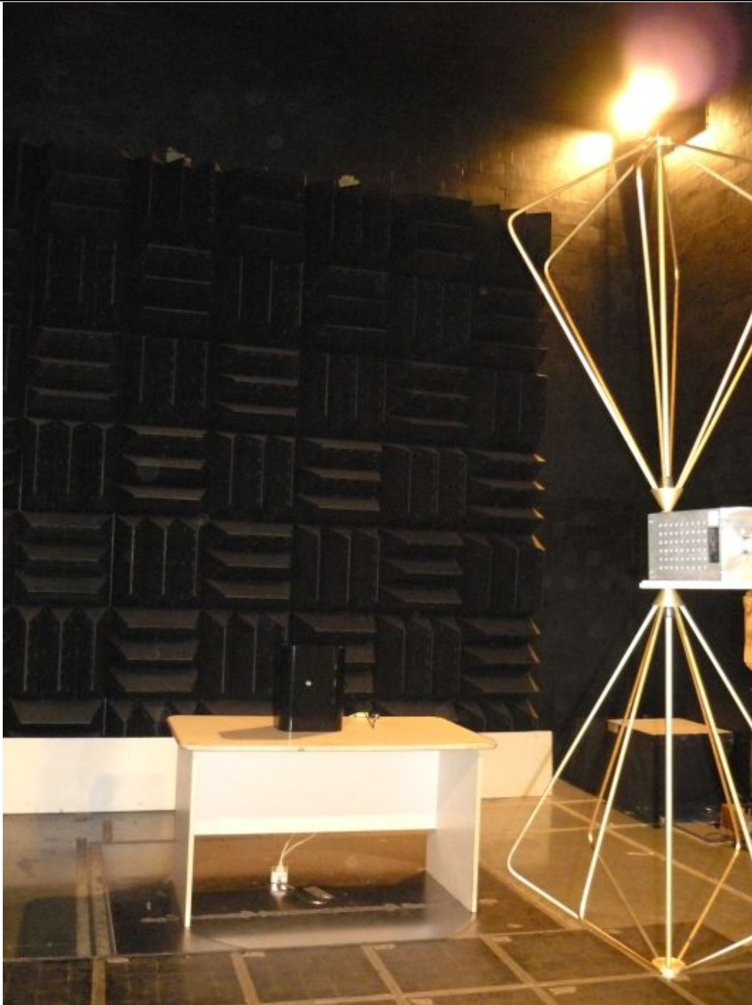
Fig. 15 4 Radiated Susceptibility Test Setup inside Semianechoic Chamber
