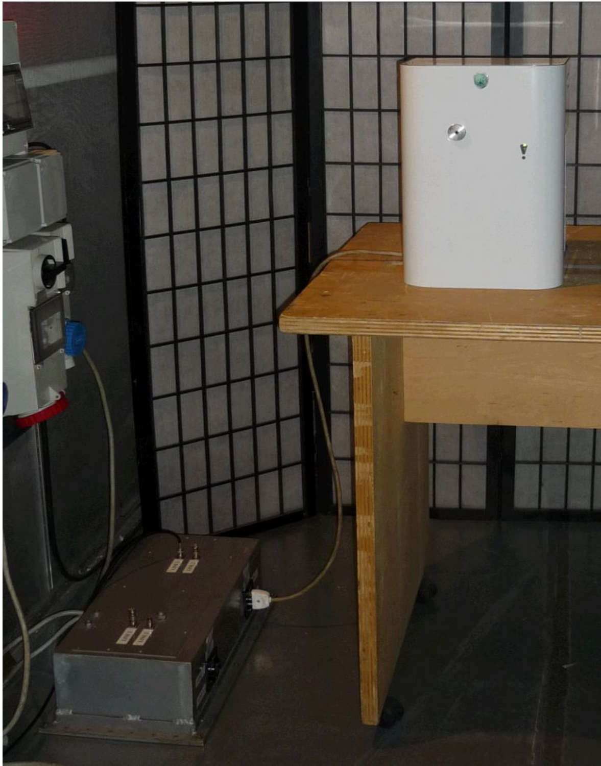
Fig. 15 5 Conducted Emissions Test Setup
